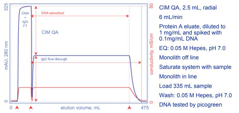
This experiment was conducted to determine the ability of a monolithic anion exchanger to remove DNA when IgG is present in the sample. DNA levels in the eluted IgG were less than 1 ng/mL (limit of linear detection for picogreen) at all sampling points, indicating at least 5 logs of removal. DNA levels in commercial IgG preparations after 2 purification steps are usually less than 50 ng/mL.
