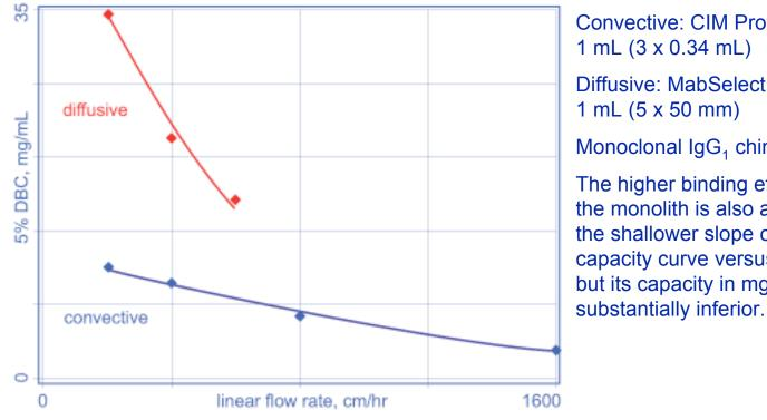
Convective: CIM Protein A HLD, 1 mL (3 x 0.34 mL) Diffusive: MabSelect Xtra, 1 mL (5 x 50 mm) Monoclonal IgG<sub>1</sub> chimera The higher binding efficiency of the monolith is also apparent in the shallower slope of the capacity curve versus flow rate, but its capacity in mg/mL is
