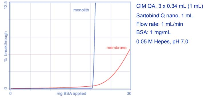
Binding capacity for host cell proteins is usually the limiting factor in determining the size of the anion exchanger. In this example, BSA is used as a model. 5% breakthrough values favor the membrane, at about 29 mg/mL versus about 21 for the monolith. However, the monolith passes no BSA until about 20.5 mg have been applied, while the membrane begins to lose efficiency after about 10 mg. Arguably, this makes the monolith the more effective candidate, especially given its higher DNA capacity.
