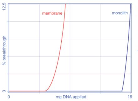
Sartobind<sup>™</sup> Q nano, 1 mL CIM QA, 3 x 0.34 mL (1 mL) 1 mL/min DNA: 1 mg/mL Sample and media equilibrated to 0.05 M Hepes, pH 7.0
